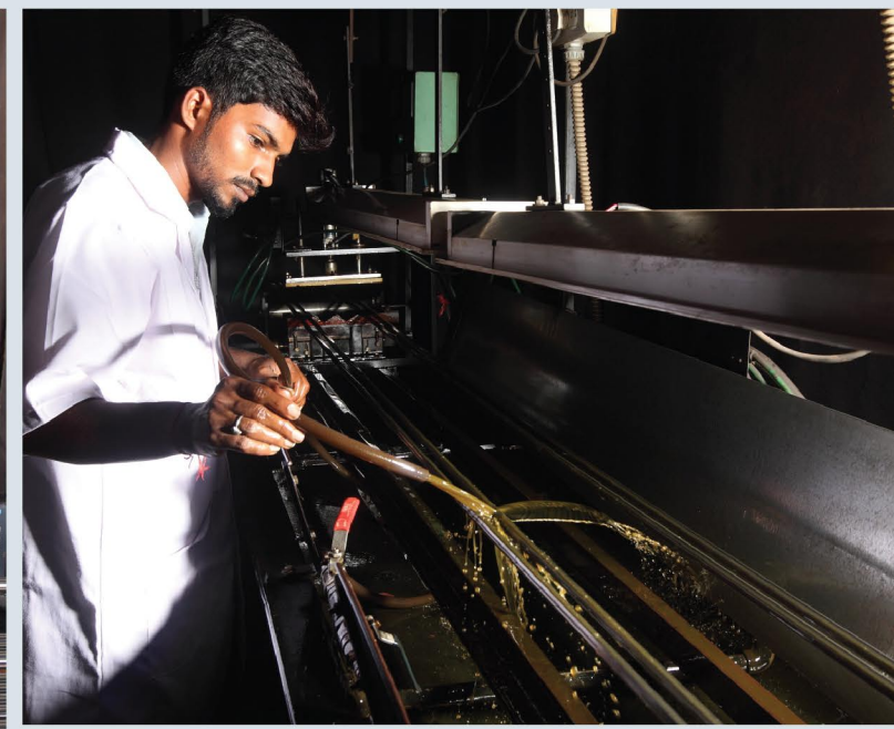
MPI under UV light for crack detection
